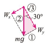
$$mg : W_y = 2 : \sqrt{3} \quad 2W_y = \sqrt{3}mg \quad W_y = \frac{\sqrt{3}}{2}mg$$
