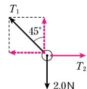
$$T_2 = T_1 \sin 45^\circ = 2.0\sqrt{2} \times \frac{1}{\sqrt{2}} = 2.0\text{N}$$
